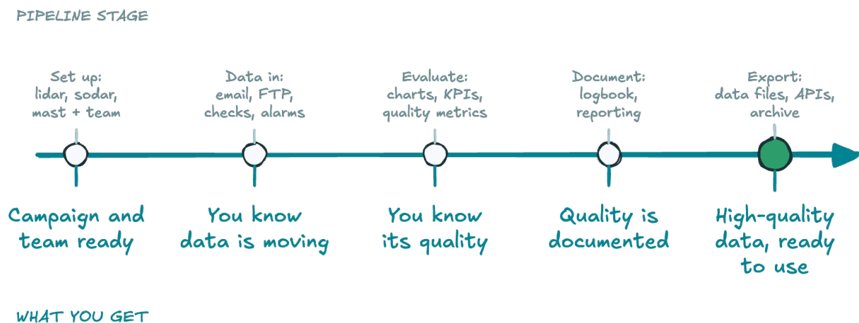
Figure 1 The five stages of an effective wind data monitoring pipeline, and what each one gives you
